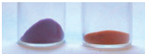
Figure 1. Color change of silica gel supported 1 upon CO ligand exchange in the presence of air containing 50 ppm CO (picture courtesy of the authors). [7]
